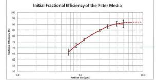
Test data: Ralative Humidity: **53,3%** Temperature: **19,7°C** Ambient pressure: **1009 hpA** Air Flow: **304,1 m<sup>3</sup>/h**  Filter flow rate: **90cm/s** Test dust: **SAE A4Coarse** Dust Concentration: **17,9 mg/m<sup>3</sup>** Corona off/on: **off** No. of repeated measurements: **3**
